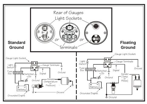
**Diagram D**Temperature/Pressure Gauge Wiring
