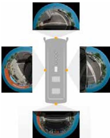
1\_ Installed cameras enable the driver to see 360° around the vehicle
