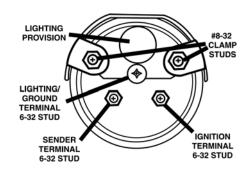
**5.** When connected, as shown, the pointers move when power is applied.
