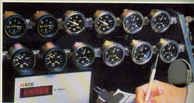
Gauges and tachometers are statistically selected from production lines and inspected for accuracy during thousands of test cycles.
