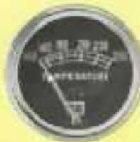
442412 Safety Water Temperature Gauge has 48" tubing and 1/2" P.T. connection. 72" and 144" tubing also available. 2-1/32" dia. case with chrome bezel.
